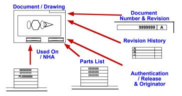
When a change is applied to a product (or component of a product), its descriptive configuration documentation (engineering drawing, product model) is updated to reflect the change. The unique identifier assigned to a product, or part, and the marking on the part itself, are changed to distinguish one configuration of the product from another, when:
