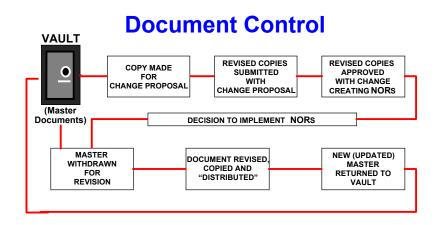
Configuration change management is essentially a process for managing baselines. Baselines are tools to match the need for consistency with the authority to approve changes. A configuration management system or plan must recognize:
