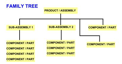
The product structure shows the top-down relationships among the various parts that make up the product and the quantity of each. The product structure is complete when all parts are included.
