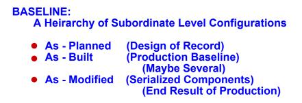
Baselines are the fundamental foundation of CM. Baselines provide an assurance of the stability and consistency of information needed for subsequent activities. They provide a common communication of product definition and also a vehicle permitting transfer of authority over all or a portion of a product's definition. The requirements definition established before beginning a product's design represents a baseline; the completed detailed drawings, as production begins, represents another.
